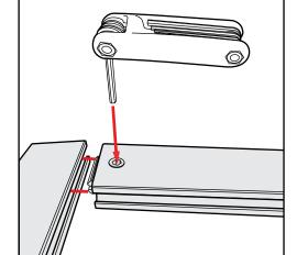
**Extrusion & Lock Connection**
