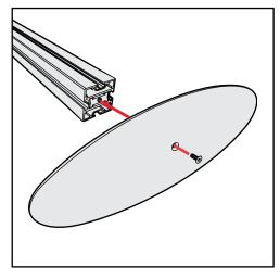
Base Plate & Extrusion Connection
